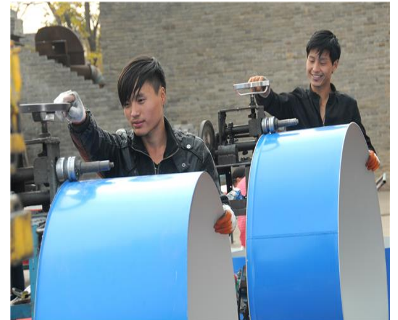
仓体生产 production of the silo's main body
