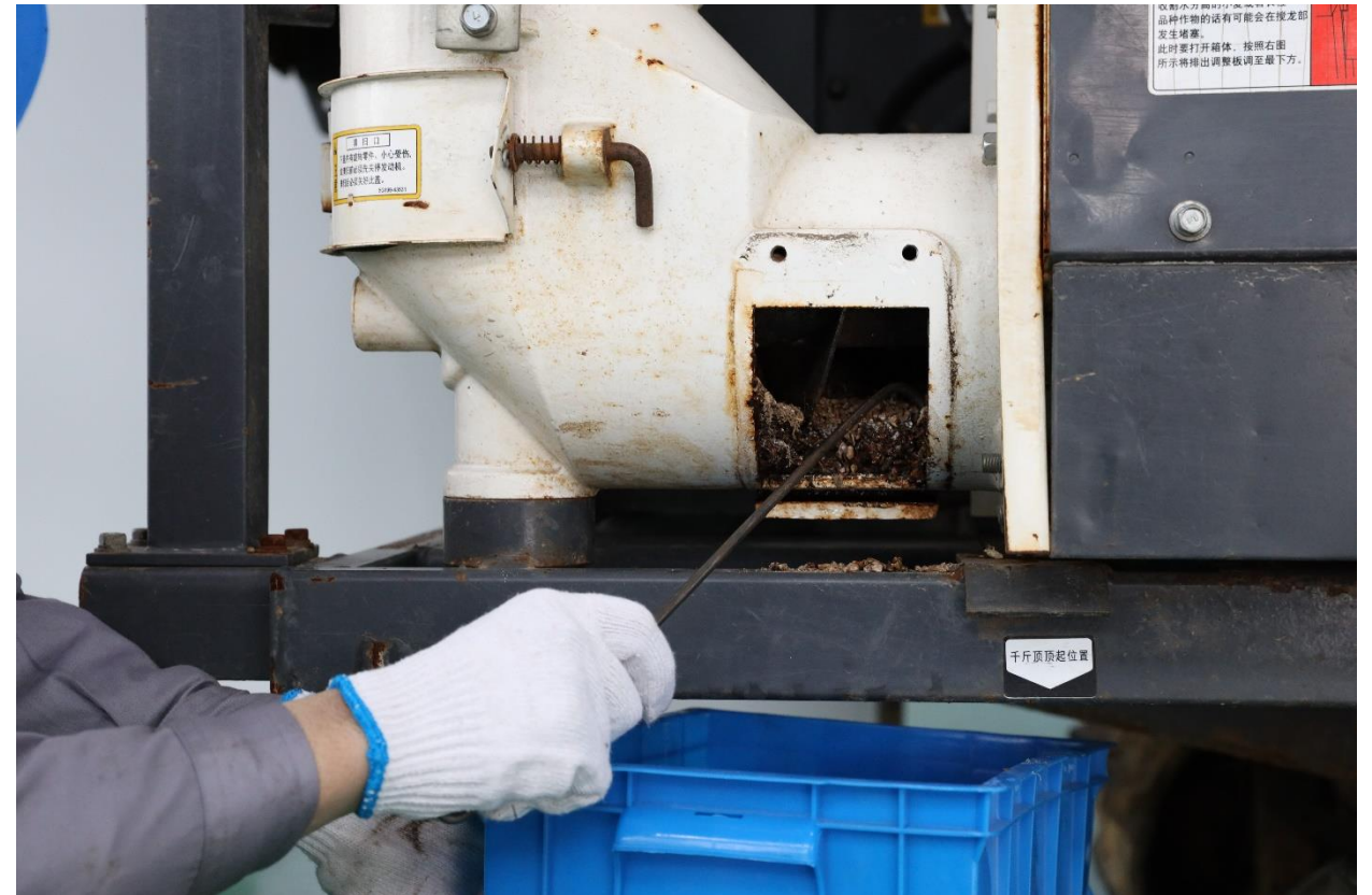
grain discharger cleaning
