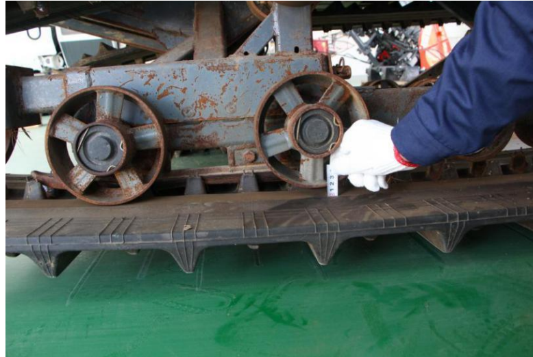
Check clearance between the 4 th wheel and the track
