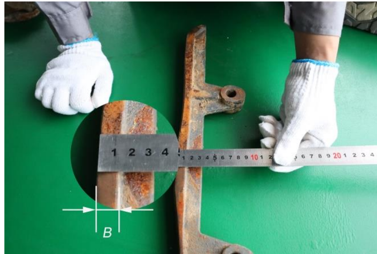
2-15b check track rail
