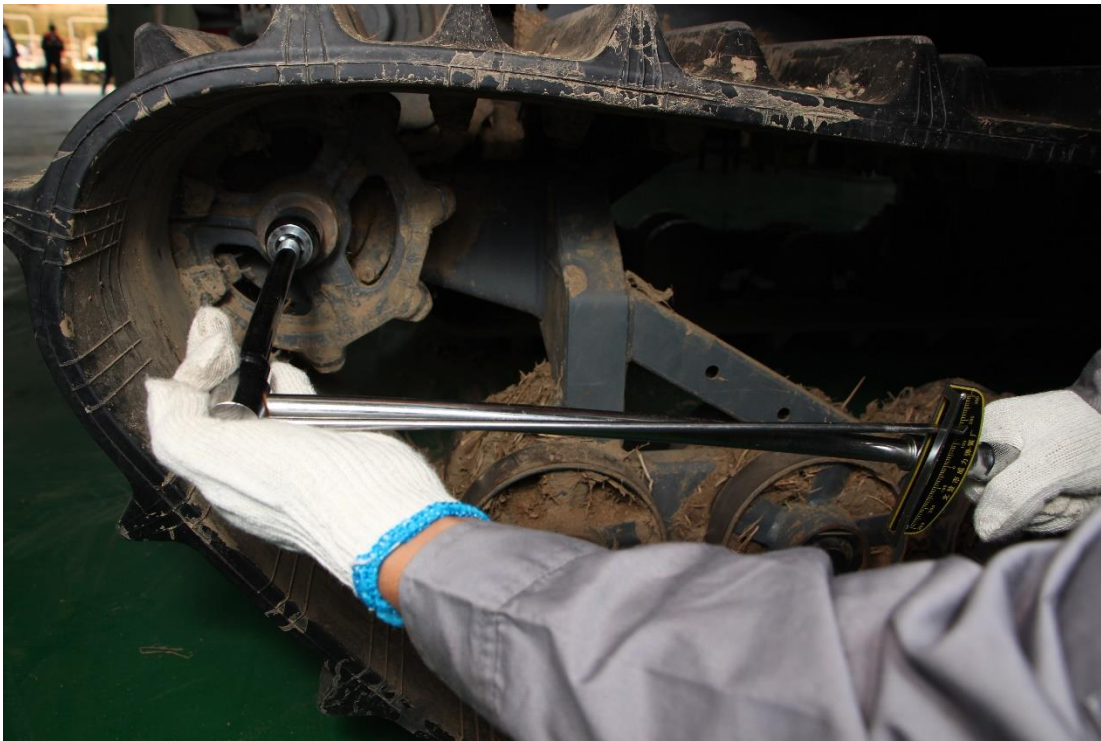
driving wheel bolt fastening
