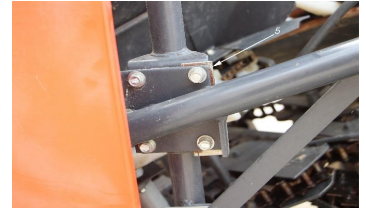
3. Guide rod mounting bolt; 4. Guide bracket
