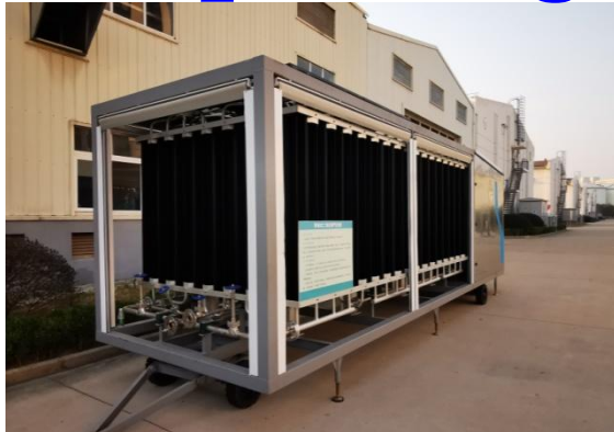
CO 2 gasification unit
