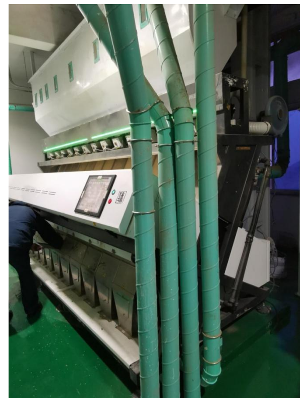
回砮谷净化设备 Equipment to separate brown rice from rehubrang paddy
