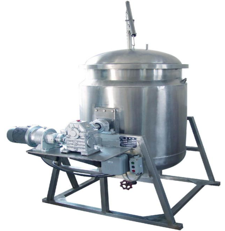
蒸煮筒 cooking cylinder
