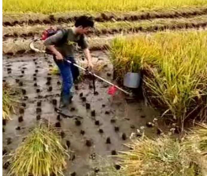
Backpack windrowers cut down rice and stack it in an orderly manner
