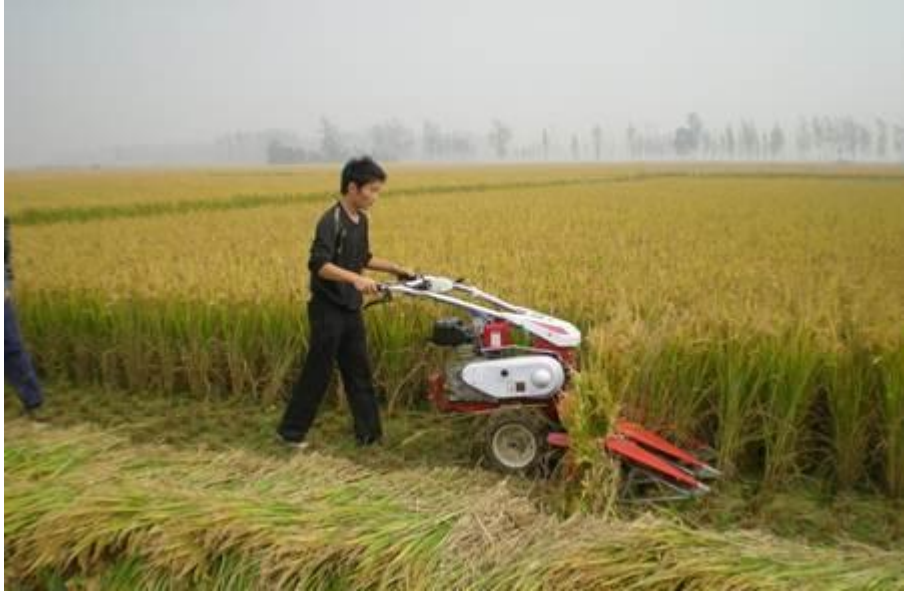
Handheld windrower cuts down rice and stacks it in an orderly manner
