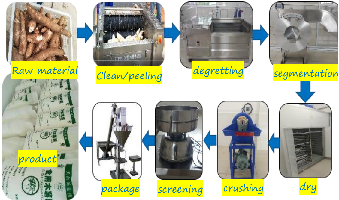
Dry processing Technology of Cassava Powder
