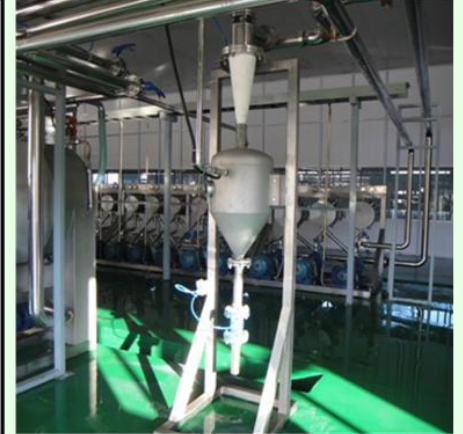
3. Tuber rasping 4. Cyclone de-sanding
