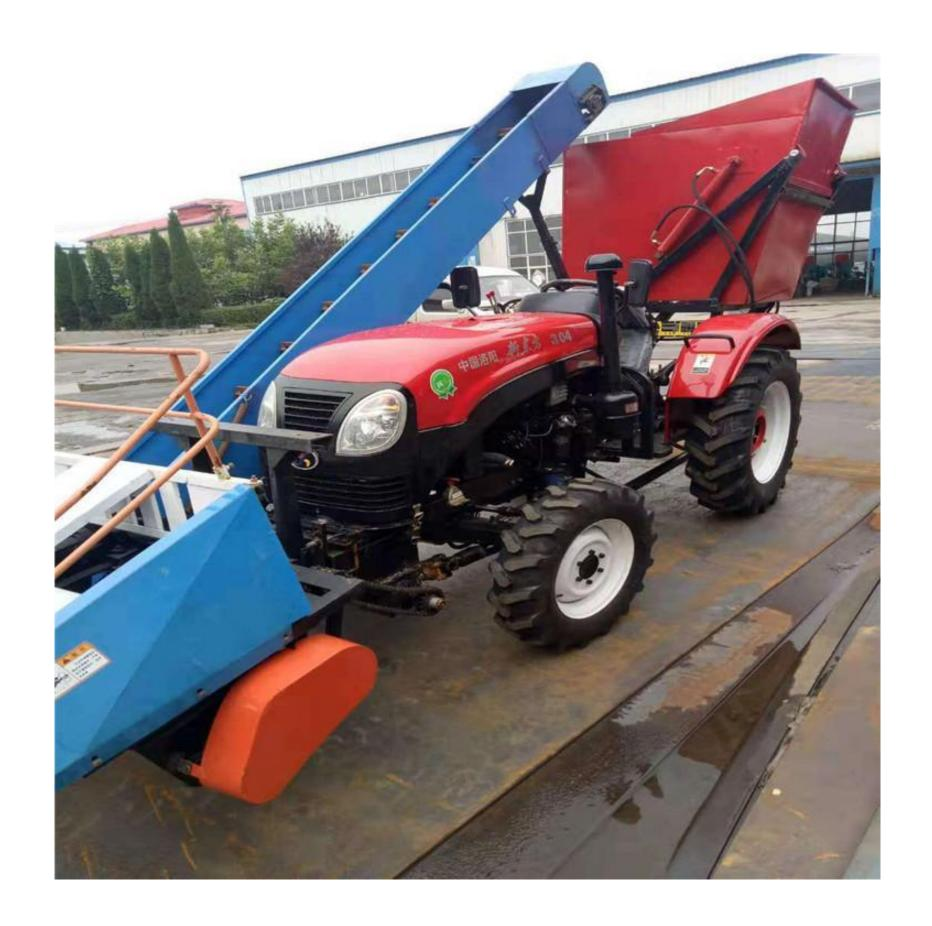
悬挂式收获机(需配套动力) knapsack harvester (supporting power required)
