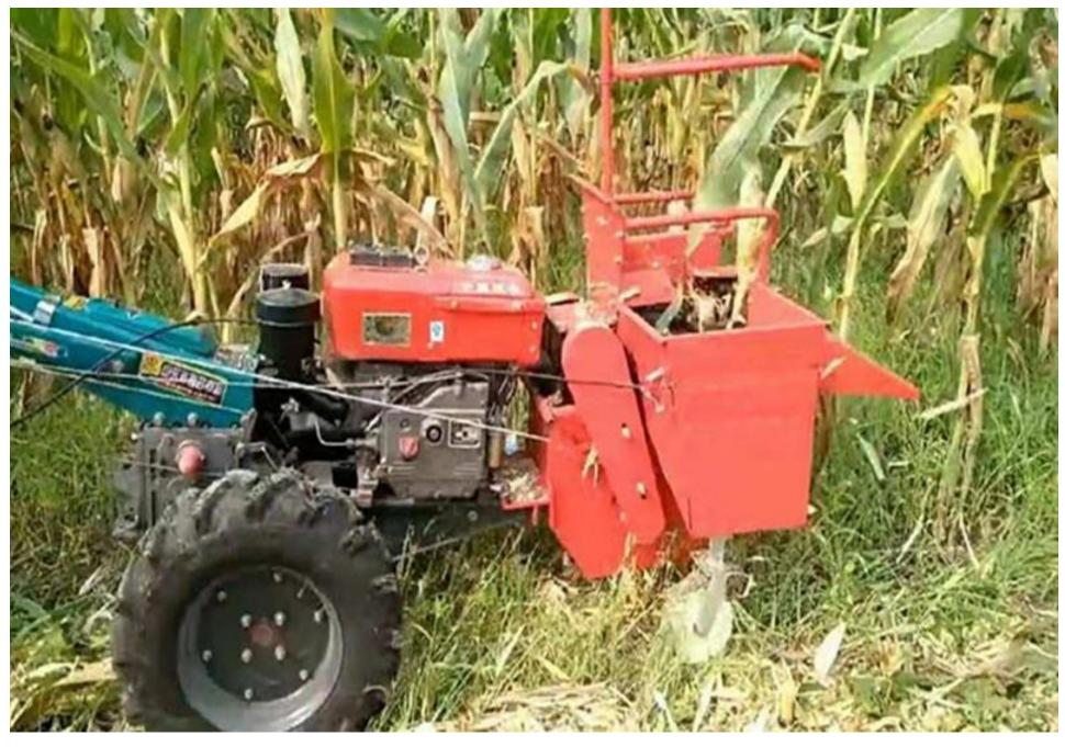
手扶自走收获机 hand-held self-propelled harvester
