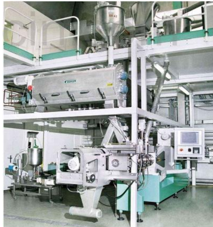
The Buhler extruder used in the NutriRice process. Photos courtesy of Buhler.
