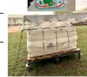
Anti-CO 2 permeable anti-mould hermetic storage system
