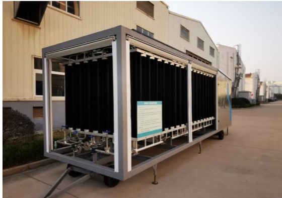
CO 2 gasification unit
