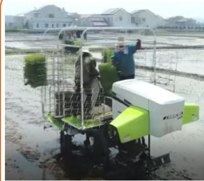
中联重科2ZPY-13A水稻有 序抛秧机 Zhonglian 2ZPY-13A rice seedling throwing machine
