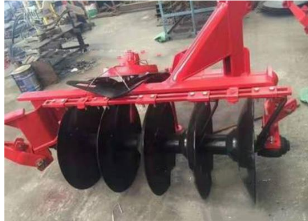
FZ-12驱动圆盘耙 FZ-12 drive disc harrow
