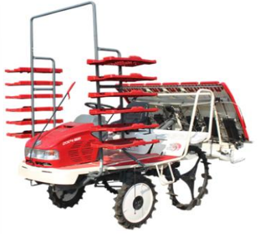
2ZGF-6/6A高速乘坐式 插秧机 2ZGF-6/6A High-speed riding rice transplanter
